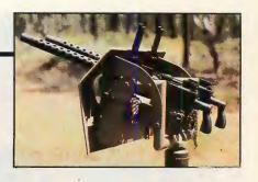
Flexible twin mounting of MG4 AA. Now firing from open bolt position, this 7.62x51mm NATO caliber conversion is most commonly employed on armored fighting vehicles. In this role it's as good as it ever was — and still better than most.
